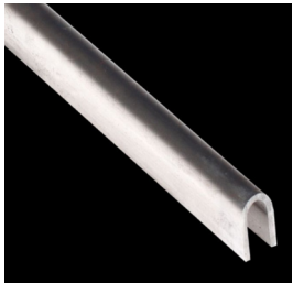
U-Edging, Carbon Steel, Hot Rolled, 14 Gauge (.0747" Thick), Type 450 U-Edging (1/2" Opening x 1" Width)
